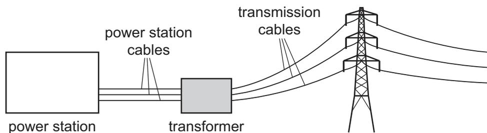
How do the voltage of the transmission cables and the current in them compare with their values for the power station cables?
